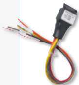
RY-24L Form C Door Release Relay
